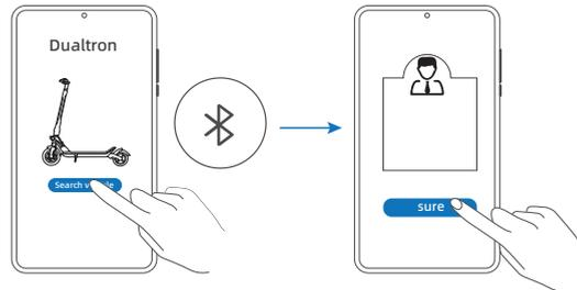
Click "Search vehicle" and pair with your scooter. \* The scooter is connected to the Dualtron app when the Bluetooth symbol lights up.
