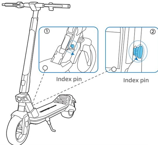
Unlock the folding handle by pulling the index pin outward.
