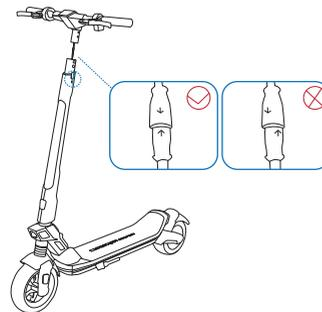
Connect the cables by aligning the arrows.
