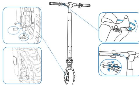
Adjust the brake cable to the appropriate position and tighten the screws.
