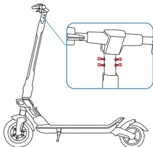
Attach all four screws without tightening them. Once all screws are attached, tighten them.
