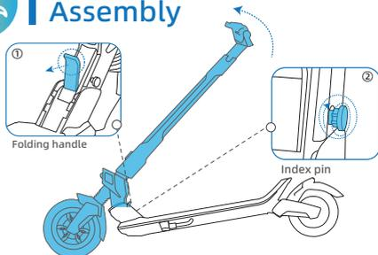
Pull the handle outward and lift the steering tube until fully extended.
