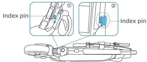
Pull the indexing pin outward to unlock the folding handle.
