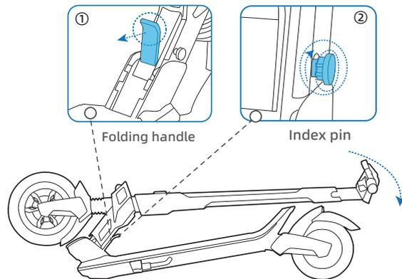
Pull the folding handle outward and slowly put steering tube down. Please remember to insert the index pin back to lock the folding.
